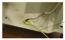
Wire to be connected to the ground
